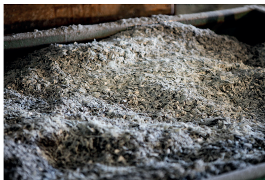
Elium® composite waste before compounding. Courtesy of Arkema, © Maxence Peyras
