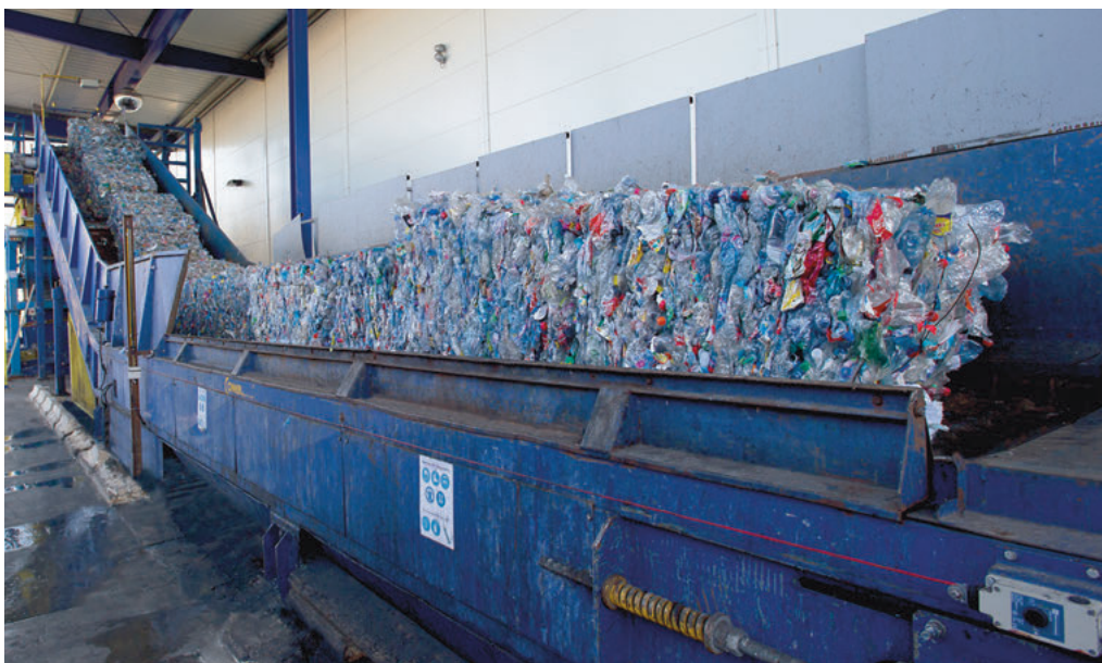
Depackaging machine for bales containing collected plastic bottles, Usine France Plastique Recyclage, Limay Photo Credits: SUEZ
