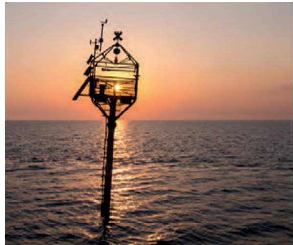
Automatic oceanographic platform in the Gulf of Trieste. ©Shutterstock
