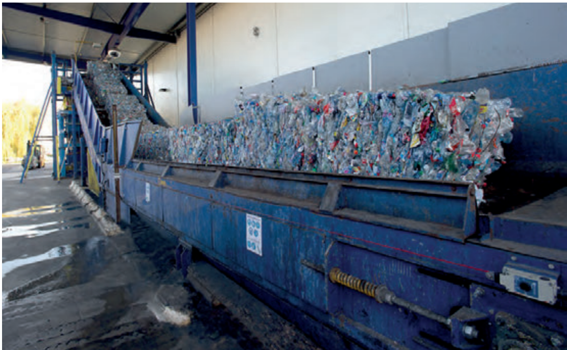
Deconditioner for bales containing collected plastic bottles - SUEZ Plant – France Plastic Recycling – © SUEZ / MH productions / Philippe Mencia.
